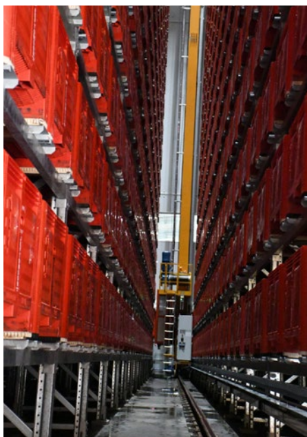
Thousands of bins of fruit can be stored in the automated retrieval system at Redland Premium Fruit at Mooroopna. Only robots operate in the dark and cold atmosphere of the tower.
