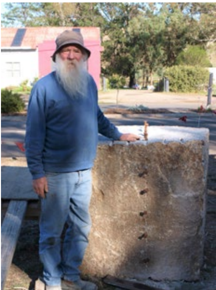
David Pratt stands next to the 3 tonne rock which has been drilled and had plugs and feathers placed in in, ready for splitting.
